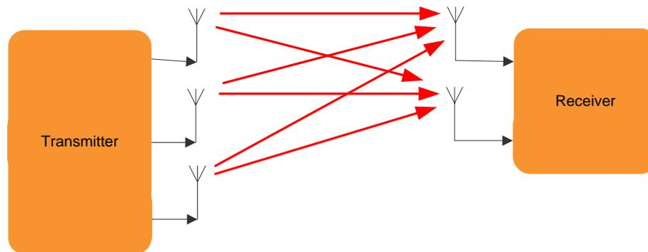
Figure 9: Multi-Antenna System Example
